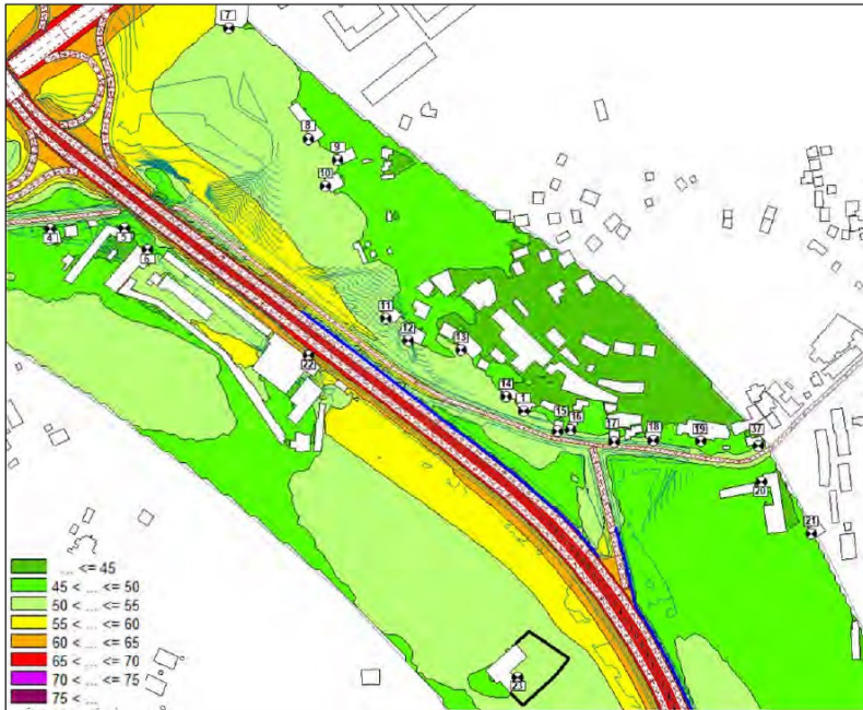
Figure 21 : Noise map calculated at 2m high – Situation 2021 with project, with noise barrier (v2) – Night period – West area
