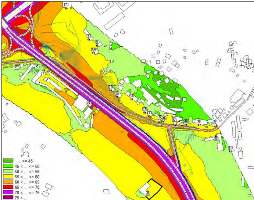
Figure 16 : Noise map calculated at 2m high – Situation 2021 with project, with noise barrier – Day period – West area
