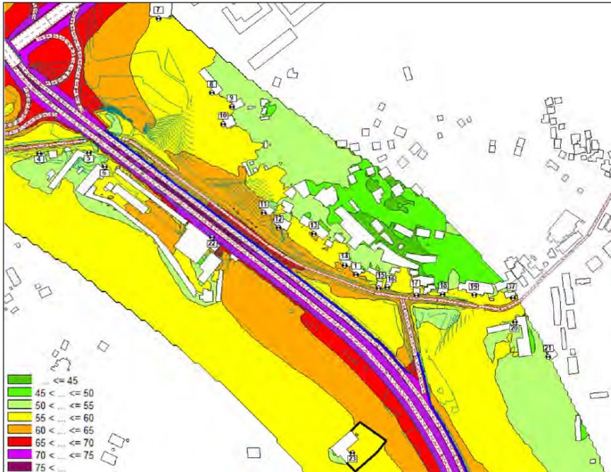
Figure 26 : Noise map calculated at 2m high – Situation 2030 with project, with noise barrier – Day period – West area
