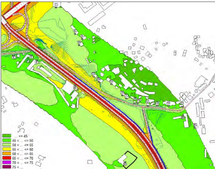
Figure 18 : Noise map calculated at 2m high – Situation 2021 with project, with noise barrier – Night period – West area
