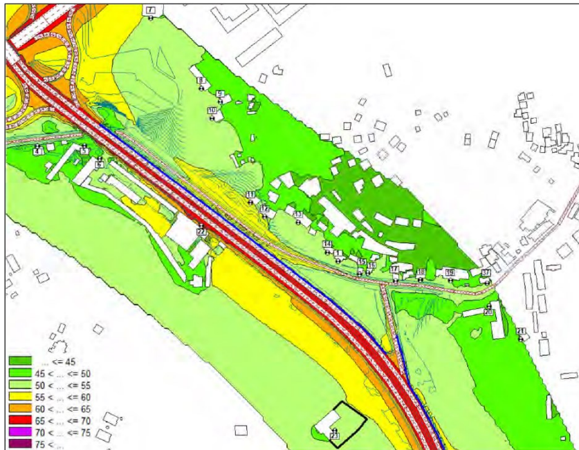
Figure 28 : Noise map calculated at 2m high – Situation 2030 with project, with noise barrier – Night period – West area
