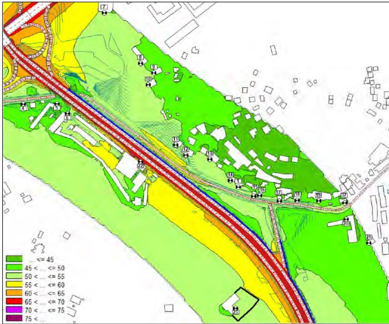
Figure 31 : Noise map calculated at 2m high – Situation 2030 with project, with noise barrier (v2) – Night period – West area
